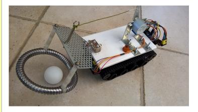
Progress has been made last week on the next robot challenge - The Crazy Golf. So the idea is to push or trap a golf ball around a course having ramps, rockers, and other nasty objects to navigate, before depositing the ball up a ramp and into the ball drop bucket. The photo shows the 2019 course.
