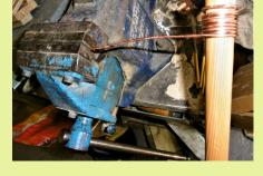
I then drilled a hole through an old broom handle. After anchoring the end of the wire in the hole, I wound the wire around to make a coil. My first attempt wasn't brilliant as you can see, but I got better each time.
