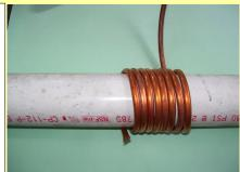
Step 2. Separate the rings. Cutters will flatten the pipe, if this bothers you, they could be sawn.
